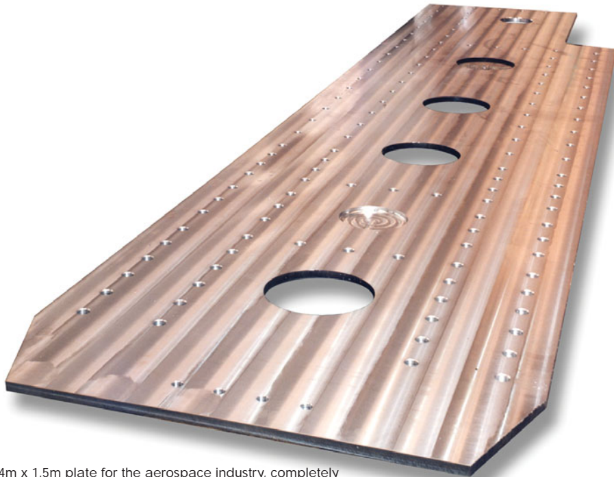
4m x 1.5m plate for the aerospace industry, completely machined in one set-up on our CNC gantry milling machine.
