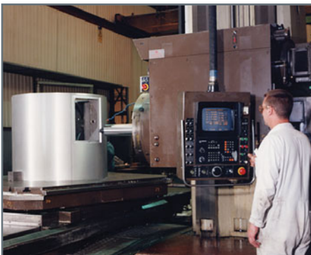
Precision machining achieved on our Union CNC horizontal boring machine.
