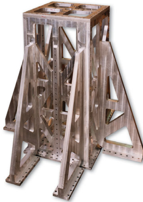
Vibration test rig for the space industry.
